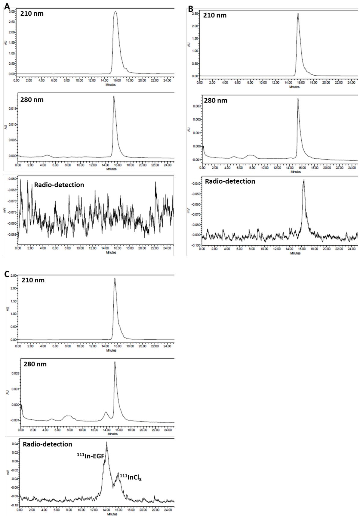
**Figure S2.** Size exclusion HPLC profiles of 0.1M sodium citrate (A),  $^{111}\text{InCl}_3$  (B) and  $^{111}\text{In-EGF}$  with excess  $^{111}\text{InCl}_3$  (C) by both UV-detection (210 & 280 nm) and radio-detection.
