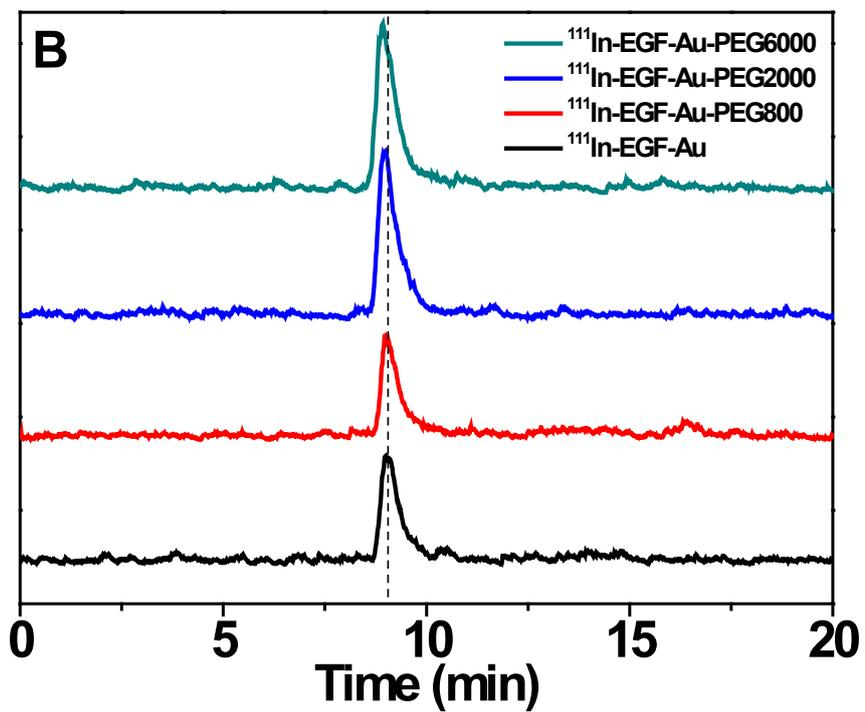
**Figure S1.** Size exclusion HPLC profiles of  $^{111}\text{In-EGF-Au}$  and three  $^{111}\text{In-EGF-Au-PEG}$  NP variants (flow rate, 0.8 mL/min) by UV-detection at 280 nm (A) and radio-detection (B), showing that non-PEGylated and PEGylated NPs were successfully radiolabelled and that EGF remains attached to the NPs after PEGylation.
