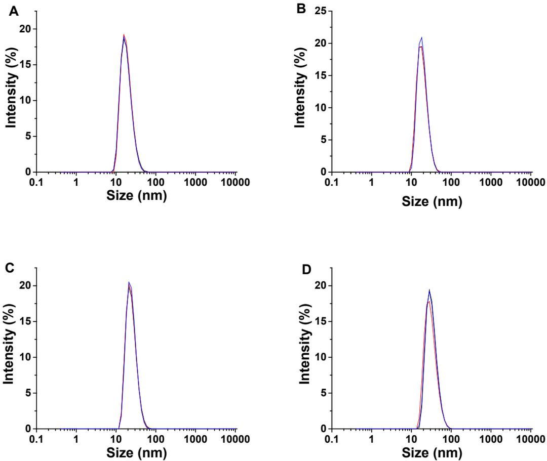
**Figure S3.** Hydrodynamic size distribution curves of DTPA-EGF-Au (A), DTPA-EGF-Au-PEG800 (B), DTPA-EGF-Au-PEG2000 (C) and DTPA-EGF-Au-PEG6000 (D) NPs from three measurements.
